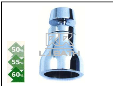
RRB - 1650 PROFILENCE wall shower c/w ball joint 1/2" 9.5 liter/min @ 3 bar
